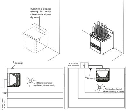
\* Recommended location of the air supply hole. Exact location may change according to the size and shape of the room.
