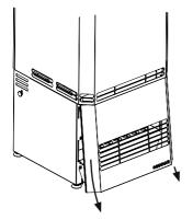
Remove the output grille by holding it slightly tilted and pulling it downwards.
