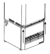
Pull from under the output grille edge outwards.
