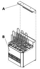
Place the cap at the connection point between the wall and the ceiling (corner) and fasten with a mounting suitable for the base material. It can be attached to the wall and/or the ceiling. Center the heater under the cap and adjust the feet so that the device is level.
